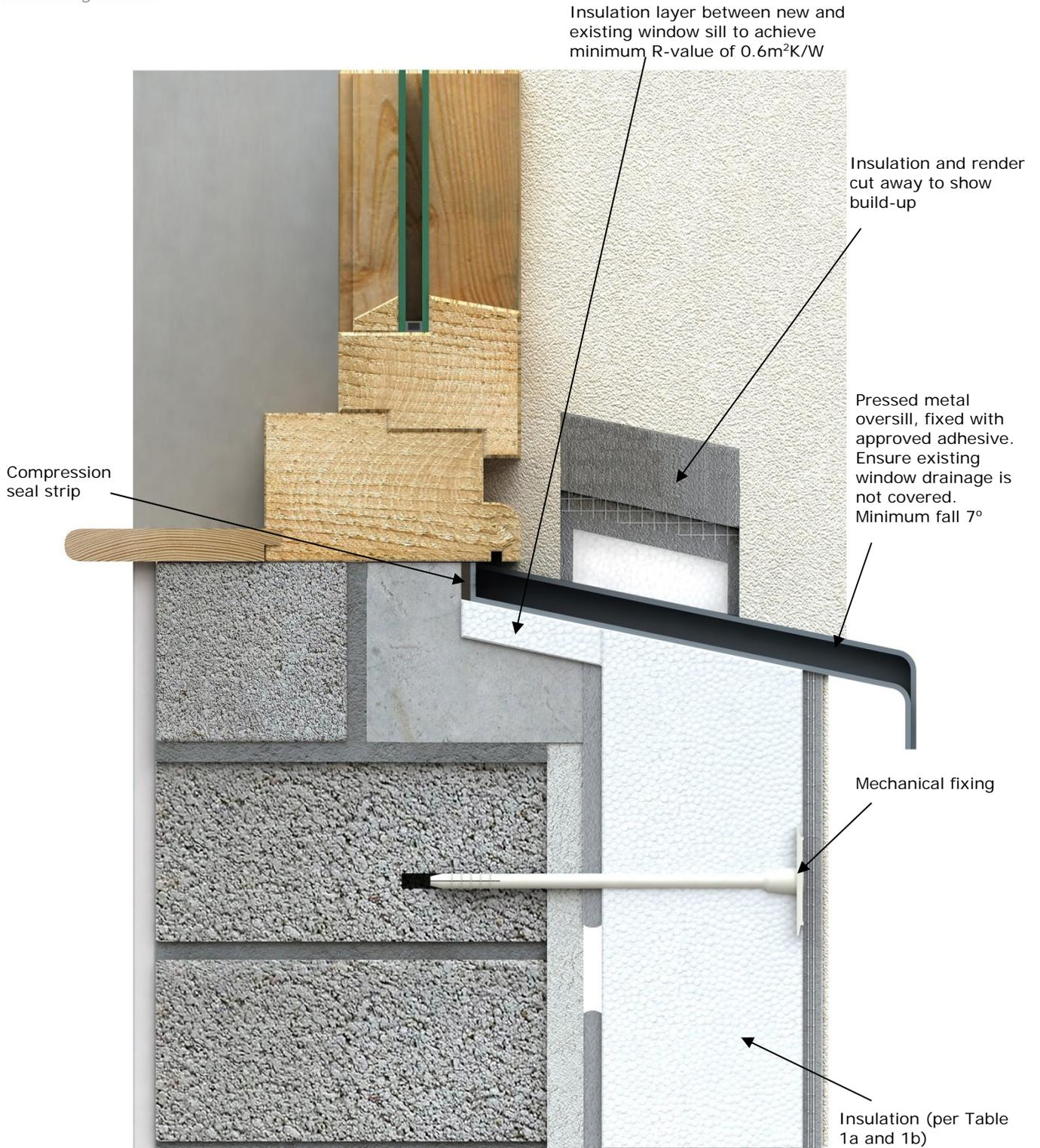
**Figure 2: Window Sill Detail**
